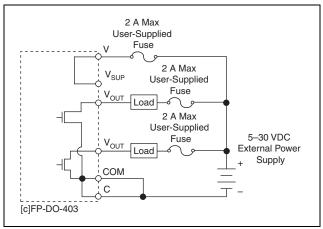
Figure 4. Wiring for High-Current Applications
